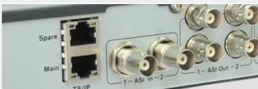
Dual Gigabit Ethernet TS/IP interface for IP based networks
